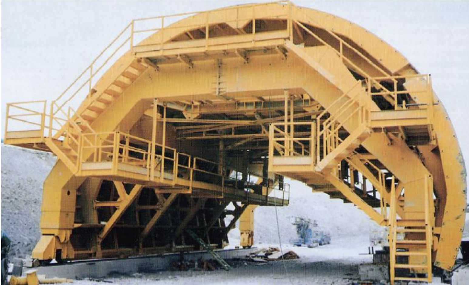
SELF- REACTING FORMWORK
