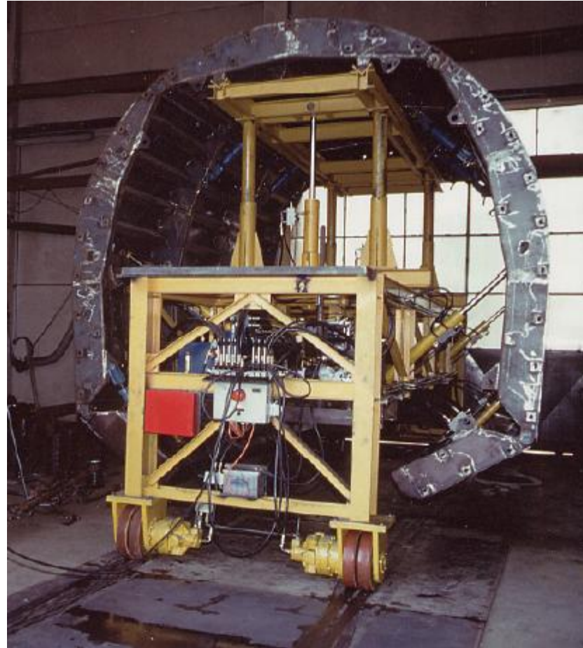
SMALL TUNNEL FORMS
