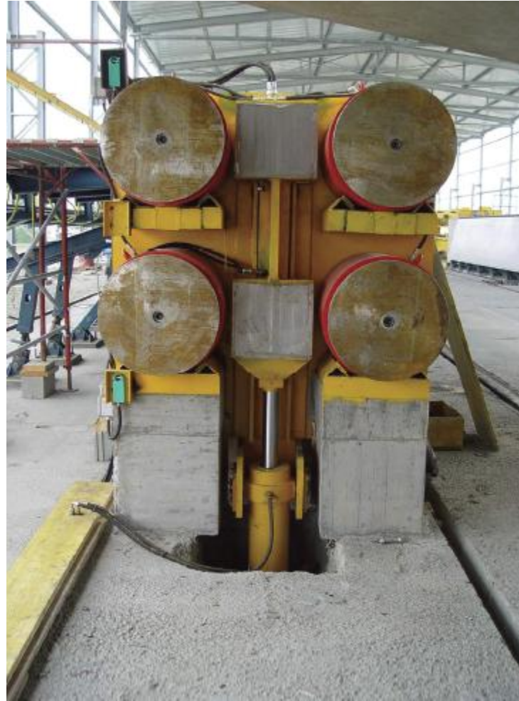
THE DETENSIONING SYSTEM
