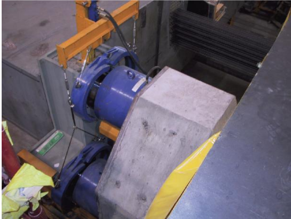
THE DETENSIONING SYSTEM
