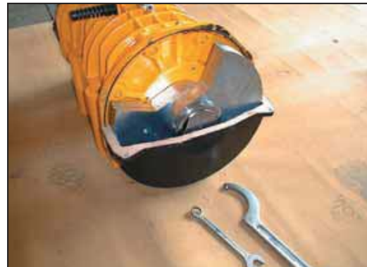
Cover in two pieces for an easy regulation of the centrifugal force with confined space.
