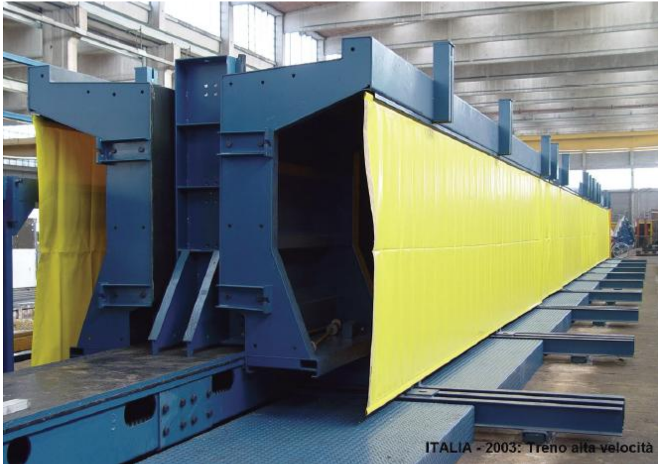
T" SHAPE BEAM CONVENTIONAL MOULD & DRAWING BACK FLANKS
