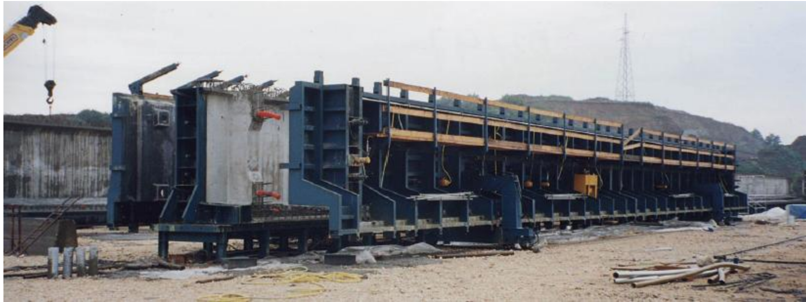
“I” SHAPE BEAM CONVENTIONAL MOULD & SHIFTING FLANKS
