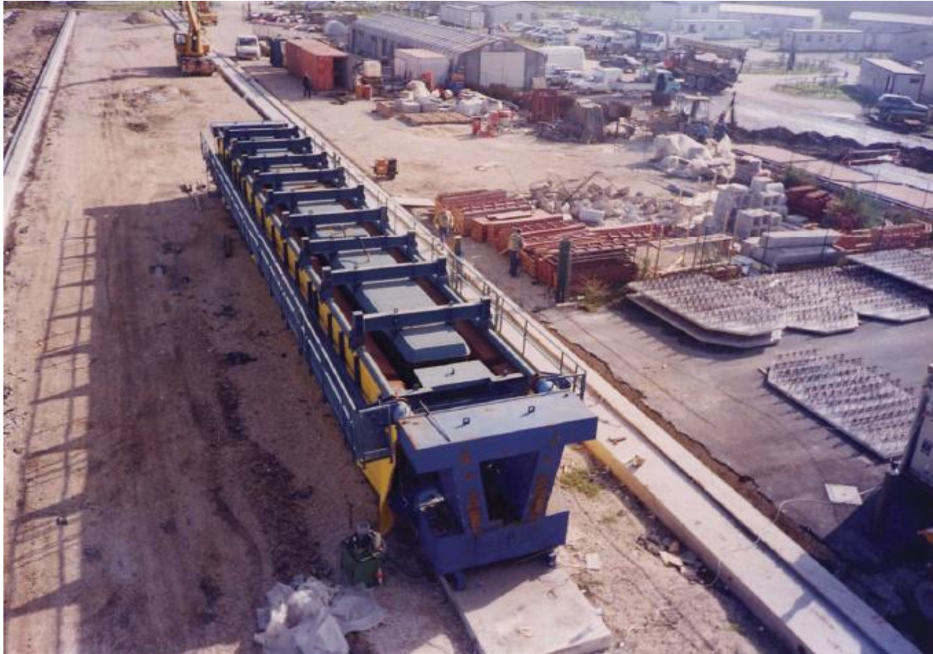
“U” SHAPE BEAM SELF REACTING MOULD
