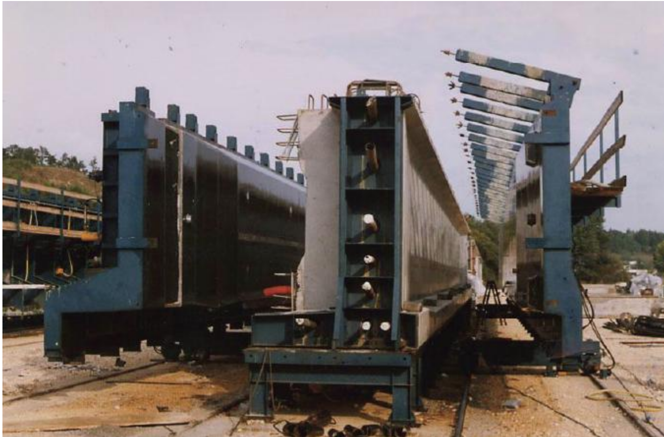
“T” SHAPE BEAM CONVENTIONAL MOULD & SHIFTING FLANKS
