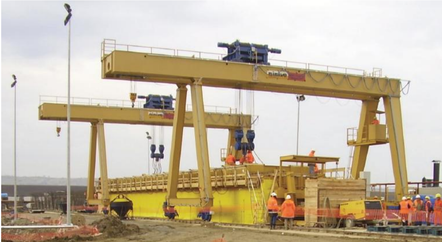
“U” SHAPE BEAM SELF REACTING MOULD
