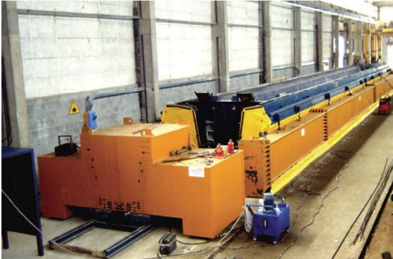
“U” SHAPE BEAM SELF REACTING MOULD
